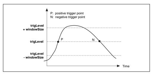
Figure 2-3. Analog Trigger Event
